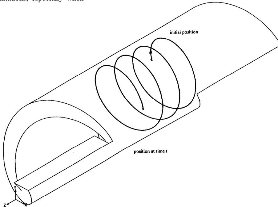
Figure 2 Particle trajectory in a single screw extruder.
